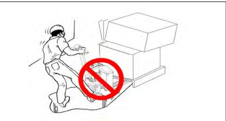
Start, stop, travel, steer and brake smoothly. Slow down for turns and on uneven or slippery surfaces that could cause truck to slide or overturn. Use special care when traveling without load as the risk of overturn may be greater. R849
