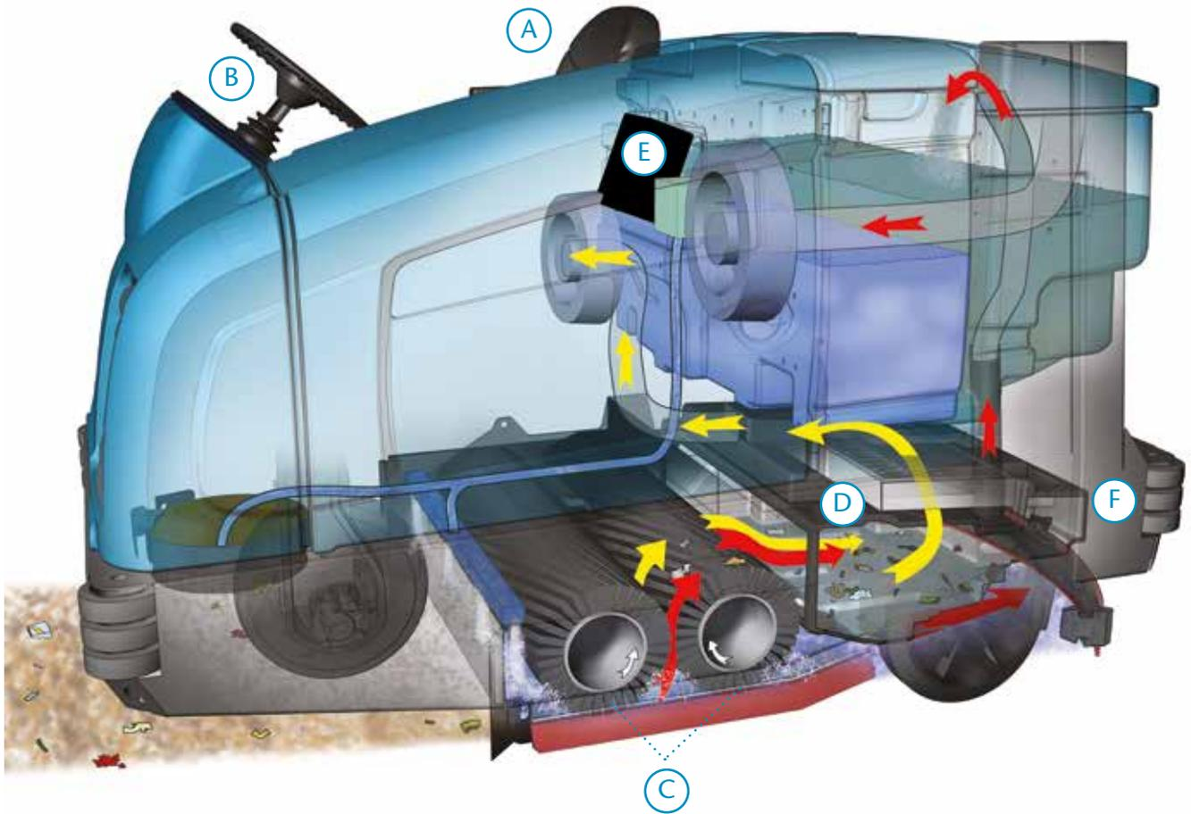
**A** Ergonomically friendly for operators, the ErgoSpace™ operator compartment makes cleaning with the M20 safe, easy, and comfortable.
