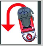
**Highly maneuverable**Turning radius 66.5" in aisles. Rear turning, parabolic squeegee and front wheel drive with 90° steering angle in both direc-
