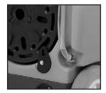
Solution gauge for monitoring amount of solution in the tank or for emptying.
